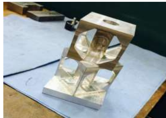
Figure 13: Show the finished machining of a cube can be run by 3, 4 and 5 axis CNC machine.
